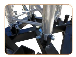
Tongue and groove joint to hinge the carriage making the assembly and the elevation easier.
