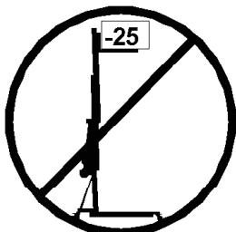
**3.15** - The minimum load to avoid problems regarding the braking mechanism is 25Kg. Without this load the brake will not work.
