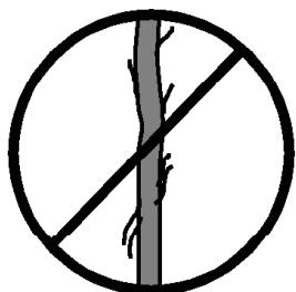
**3.12** - Before using the lift, check the condition of the cable. The cable should not have broken threads or show any signs of crushed/flattened areas. NEVER use faulty cables, always change them if there is any doubt. Only use VMB steel cables; reference: DIN 3060.
