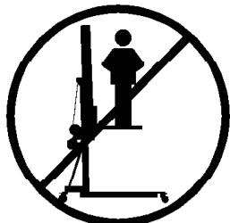
**3.1** - The TE-034 is a machine designed to elevate loads upwards in a vertical direction, It should NEVER be used as a platform to elevate people.
