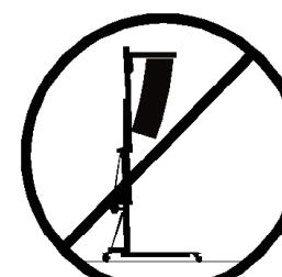
**3.4** - This lift should NEVER be used to elevate a load that has not been properly checked. It is necessary to verify that the load is correctly supported and centred on the appropriate lift support so that the weight of the load will only elevate in a vertical direction.
